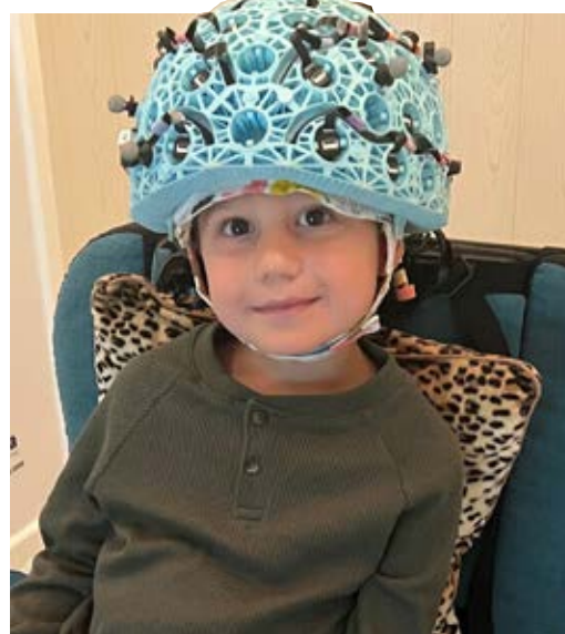
Young boy in a Cerca Magnetics quantum OPM-MEG (optically-pumped magnetometer-magnetoencephalogram) scanner. The helmet is the first wearable MEG device that will allow researchers to study the brain activity of children from birth to 5 years old. Credit: Toronto Sick Kids Hospital.
