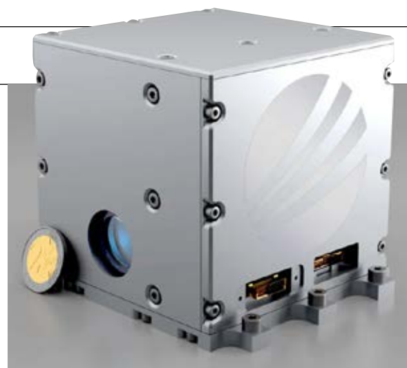
Designed for small satellites, including CubeSats in low-Earth orbit, Tesat's "SCOT20" scalable optical communications terminal offers 100 Mb/s bidirectional inter-satellite links, with a range of up to 2000 km. Credit: Tesat.
