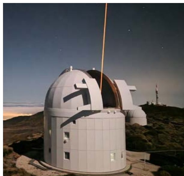
This 589nm sodium laser beam at the European Space Agency's optical ground station in Tenerife is creating an artificial star to help reveal and correct distortions in communication signals. The technology is still in the research stage. It is inspired by the proven sodium guide star technology that astronomers use to correct distortions in images caused by atmospheric turbulence. Credit: European Space Agency.
