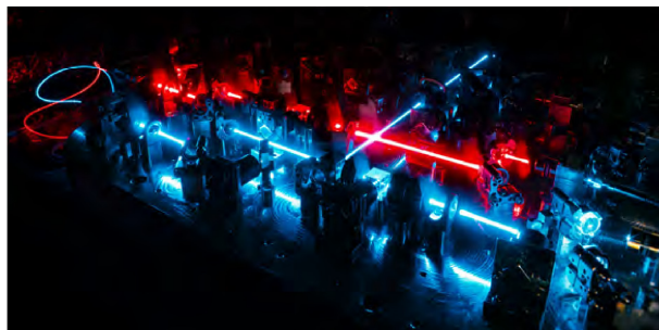
IonQ's ion-trap designs rely on a multitude of lasers and optical components. The company is now looking to scale its technology for rack-mountable deployments, partly thanks to new fiber laser systems provided by NKT Photonics. Credit: IonQ.
