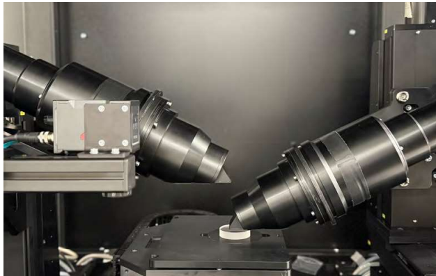
On show at the Moscone: Jenoptik's new metrology instrument, the "ImageMaster® Pro AR Reflection," which is used to measure the MTF and various image quality parameters of AR waveguides. Credit: Jenoptik.
