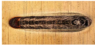
Hybrid processing for 4mm-thick copper using the 5kW blue laser (left: top view; right: cross-section view). Credit: Furukawa Electric.
