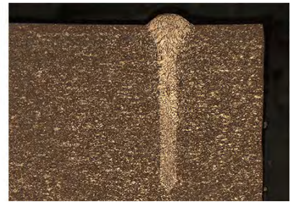
Hybrid processing for 4mm-thick copper using the 5kW blue laser (left: top view; right: cross-section view). Credit: Furukawa Electric.
