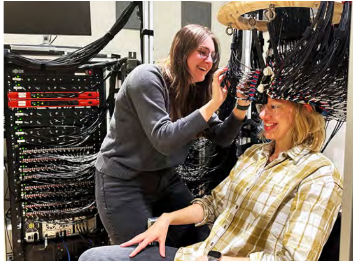
Fogarty adjusts the very high-density diffuse optical tomography (VHD-DOT) cap on labmate Wiete Fehner, ensuring optimal optode coupling and participant comfort as a critical step before data collection. Credit: Morgan Fogarty.
