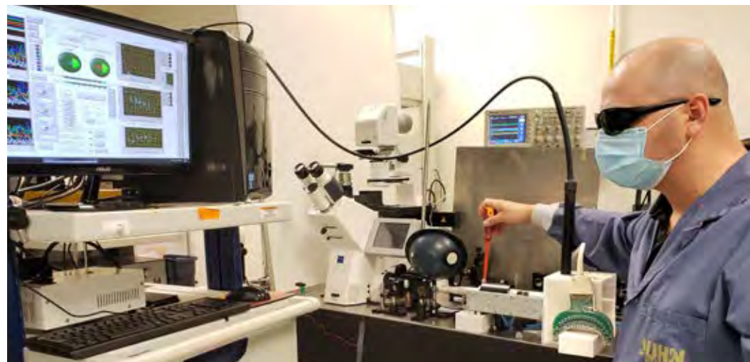
Ivan Kosik using a diffuse optical tomography system to map out the laser fluence intensity in a 3D imaging volume. Credit: University of Toronto.
