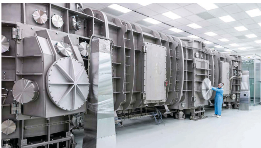
Beam us up: A newly funded research project combines the theoretical expertise of University of Rochester scientists with the theoretical and experimental capabilities of ELI Beamlines in the Czech Republic. Pictured is the compressor for generating the ultrahigh-intensity laser pulses required for the project.
