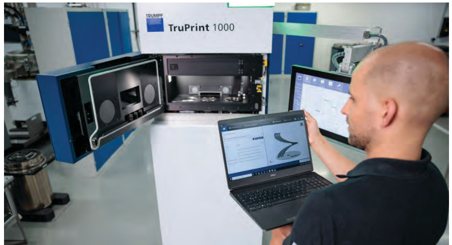
TruTops Print allows users to print parts with extreme overhangs as low as 15 degrees without requiring support structures.
