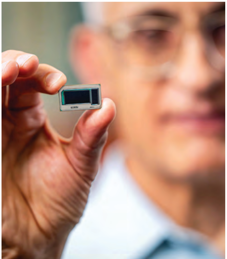
Hamid Azimi, corporate vice president and director of substrate technology development at Intel Corporation, holds an Intel assembled glass substrate test chip at Intel's Assembly and Test Technology Development factories in Chandler, Arizona, in July 2023. Intel's advanced packaging technologies come to life at the company's Assembly and Test Technology Development factories.
