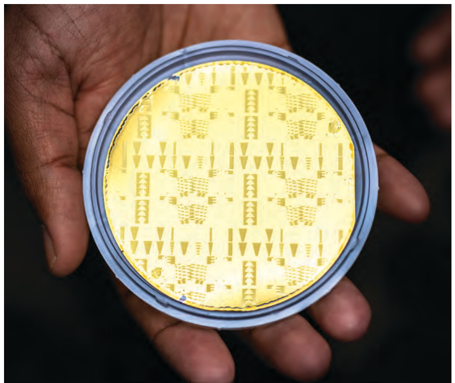
More than a thousand experimental lasers and amplifiers adorn a three-inch, gold-electroplated silicon wafer made at Sandia National Laboratories' Microsystems Engineering, Science and Applications complex.
