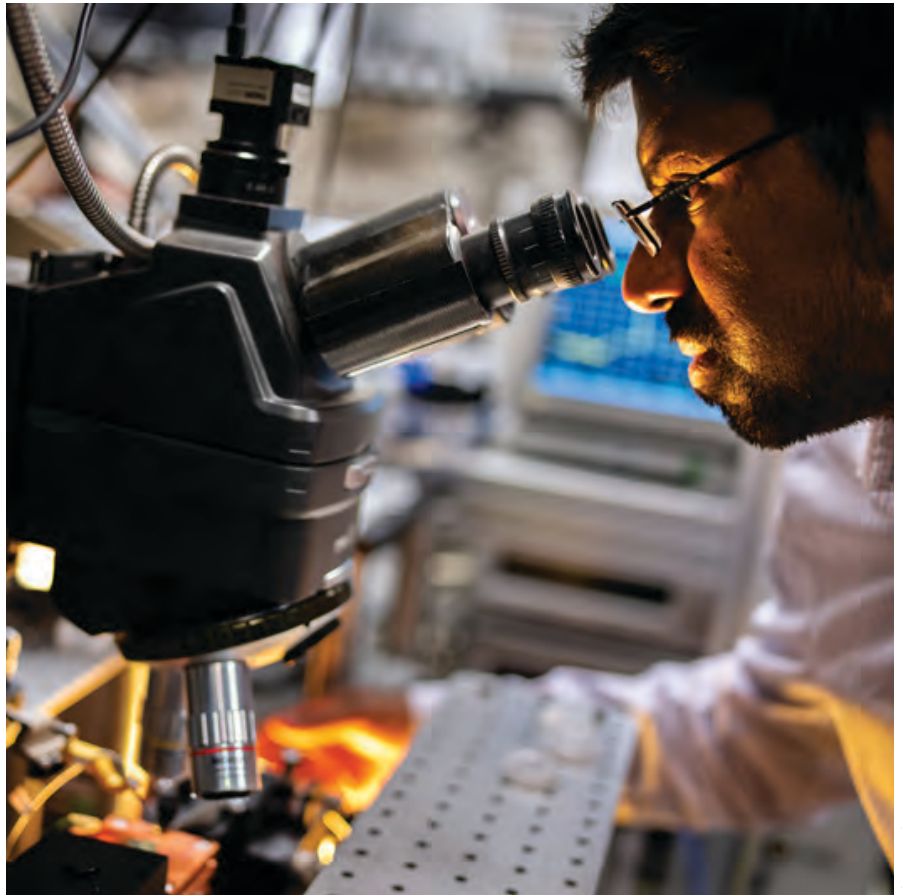
Sandia National Laboratories scientist Ashok Kodigala aligns a fiber to a chip-scale, heterogeneously integrated laser under a microscope at the MESA complex.
