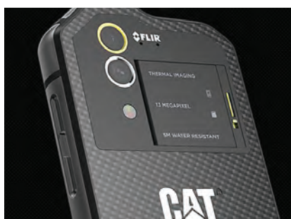
Based on Flir's Lepton core, the microbolometer-based thermal imaging camera.
