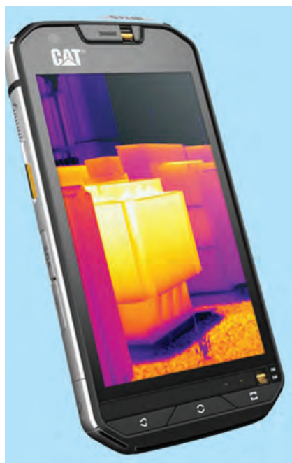
Cat S60 phone: said to be "the world's first thermal imaging Smartphone".
