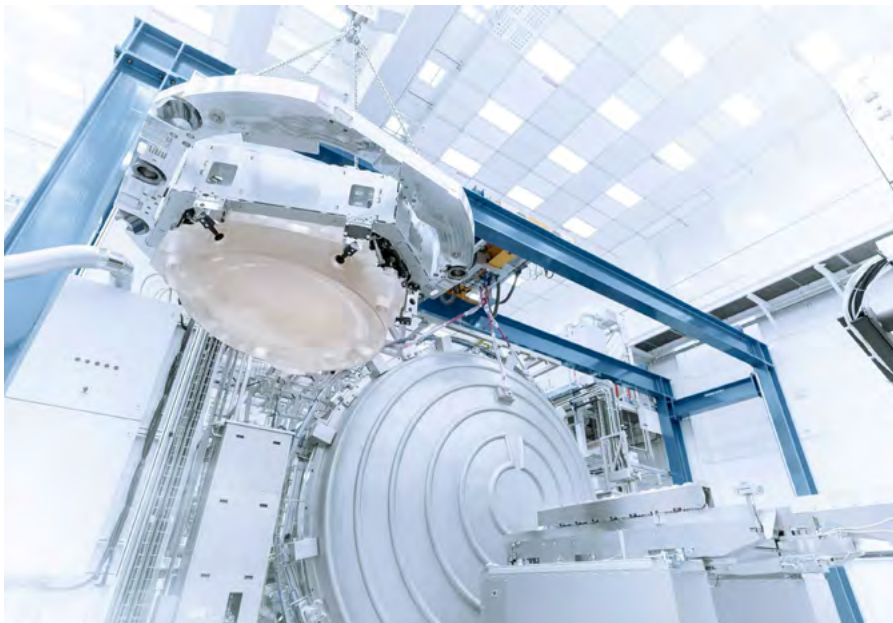
High numerical aperture (high-NA) reflective optics under development at key supplier Zeiss. Extreme ultraviolet lithography with high-NA capability is expected to be rolled out by ASML from 2025. Credit: Zeiss.
