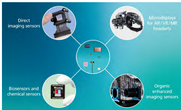
Miniaturized optoelectronic systems with emitter and sensor functions on a chip are realized with OLED-on-silicon technology. Credit: Fraunhofer FEP.
