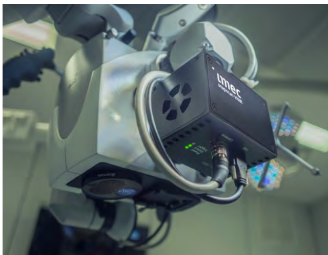
imec's "snapscan" hyperspectral camera, shown mounted on a Pentero surgical microscope made by Zeiss. Photo: imec.
