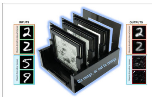
Left: Diffractive image reconstruction, in which a sequence of fabricated diffractive surfaces act on light from objects hidden behind diffusing media. Right: Images of those objects are reconstructed from the randomly scattered input. Courtesy of Aydogan Ozcan, UCLA.
