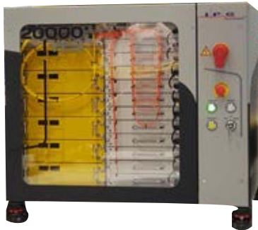
Superpower: IPG Photonics' new 20kW YLS Ytterbium fiber laser. Credit: Matthew Peach
