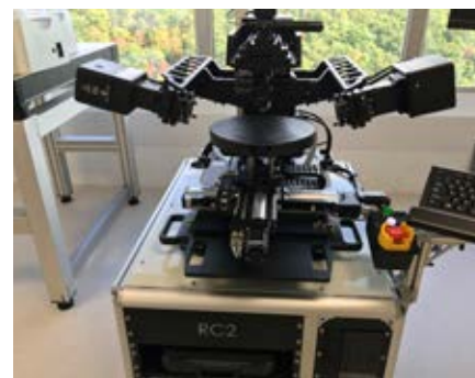
AIM Photonics’ TAP Facility Metrology Lab dual beam spectroscopic ellipsometer. Credit: Frank Tolic
