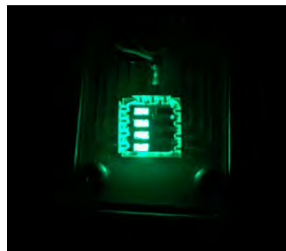
Sam Stranks' team at the University of Cambridge has produced green LEDs using CsPbBr 3 perovskite. Image credit: Miguel Anaya, University of Cambridge
