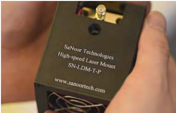
A high-speed laser LiFi transmitter developed by SaNoor Technologies allows the LiFi transmission data rate going beyond 10 Gb/s. Credit: SaNoor Technologies
