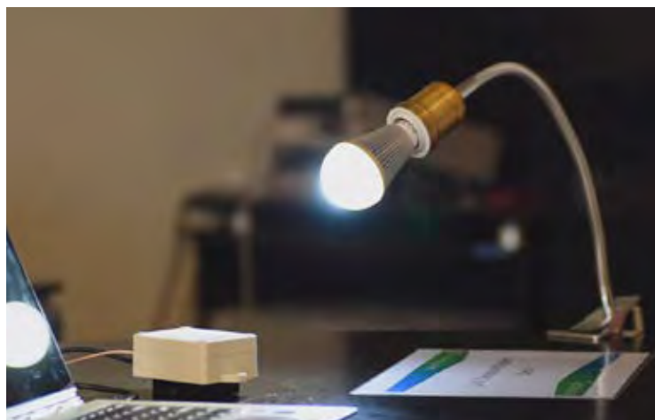
A high-speed laser white light bulb developed by SaNoor enables more than 1 Gb/s data rate LiFi communication link. Credit: SaNoor Technologies
