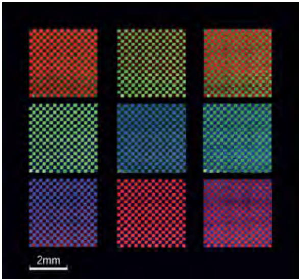
Using polarizing filters, 3D-printed perovskite nanowire LEDs enable adjustable multicolor displays. Image: N. Zhou et al., Sci. Adv. 5, eaav8141 (2019)
