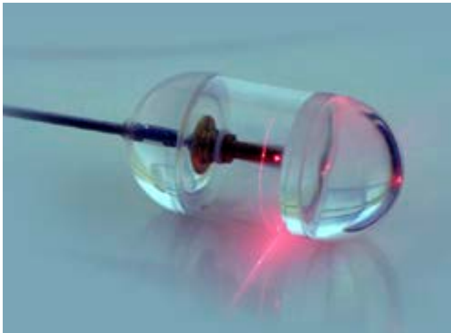
Andreas Wartak’s optical coherence tomography “pill”, for diagnosing allergy-related inflammation of the esophagus. Photo: Andreas Wartak.
