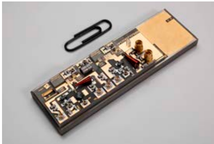
This master-oscillator power-amplifier (MOPA) laser module was launched on a sounding rocket in early 2017, to carry out the first laser-cooling experiments in microgravity. In November 2018 the German consortium that built it reported that 110 experiments were completed during its six minutes of space travel. Copyright: FBH/schurian.com.
