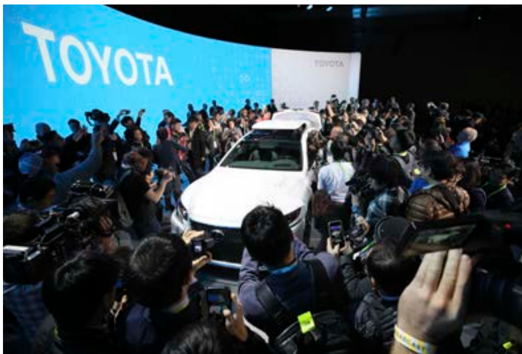
Toyota's latest "Guardian" test vehicle for autonomous driving is mobbed by the media at CES 2019 in Las Vegas. The car features high-performance lidar units in its roof section, other lidar sensors around its chassis, radar, and numerous cameras. Photo: CES.
