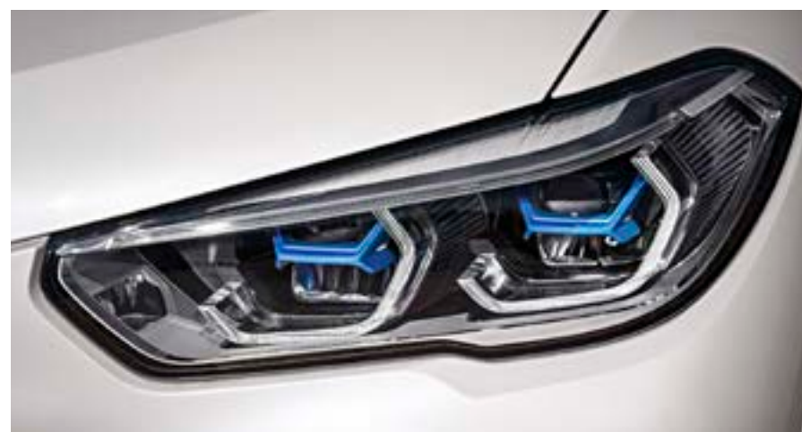
LED headlights are standard on the 2019 BMW X5, but the options list includes BMW Laserlight with adaptive LED Headlights. This technology uses a BMW Laserlight spotlight with Selective Beam, which can project a non-dazzling high beam at a distance of about 500 m. The BMW Laserlight projectors can be identified by the blue X-shaped trim inside the headlight clusters. Photo: BMW
