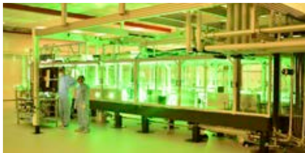
The “L3-HAPLS” beamline, which delivers petawatt-scale laser blasts at a rate of 10 Hz, was declared fully integrated and operational in July 2018. It was originally built at Lawrence Livermore National Laboratory (LLNL), before being packed up and shipped to the Czech Republic. Photo: LLNL.
