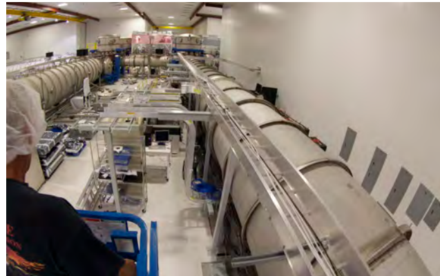
The laser and vacuum equipment area at the Hanford, Washington, LIGO facility. For the forthcoming "O3" observation run, the laser power is being increased with a new amplifier stage that will reduce fluctuations in beam pointing that has limited overall sensitivity in previous runs. Photo: LIGO/NSF.
