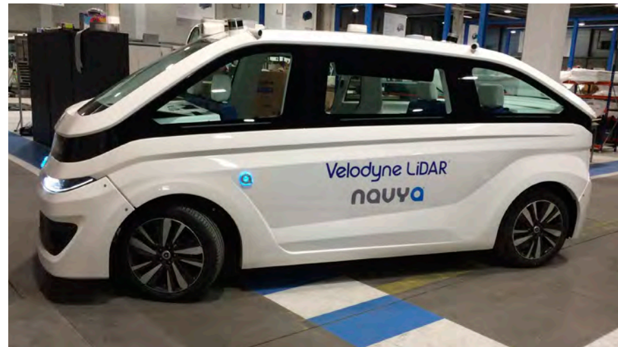
Touted for a commercial release this summer, this self-driving taxi from French startup Navya is fitted with multiple lidar units from Velodyne, alongside radar units and cameras. Photo: Velodyne Lidar.
