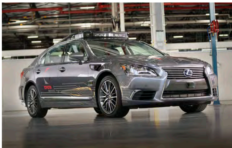
This Lexus car, fitted with a rooftop lidar system from Luminar and built by Toyota Research Institute, made an appearance at CES 2018 in Las Vegas. Photo: TRI.
