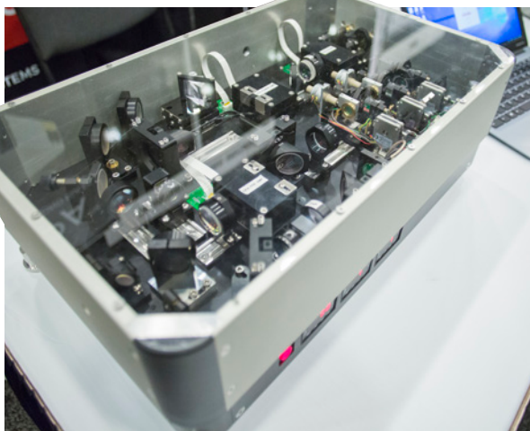
Hotlight Systems' compact source for two-photon and three-photon microscopy, unveiled at the weekend's BIOS Expo, is based around crystal technology developed at the Australian National University. Photo: Joey Cobbs.
