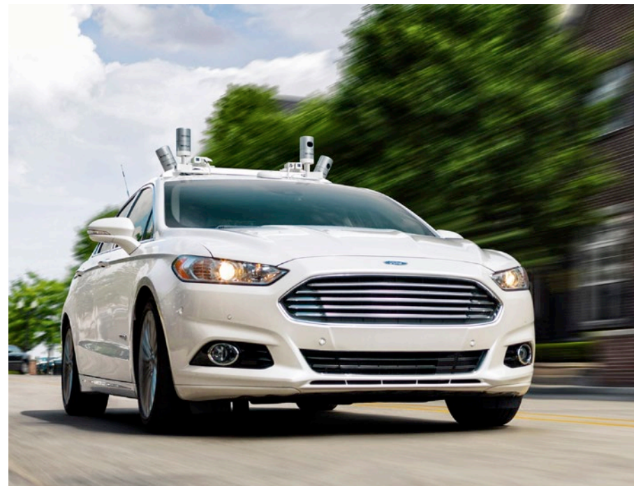
One of Ford’s autonomous vehicles, with four lidar sensors from Velodyne protruding from its roof. Photo: Ford
