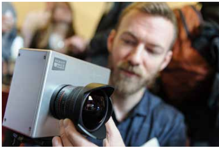
Not just any camera: this prototype imaging system, under development at QuantIC hub partner Heriot-Watt University, could aid security services with the ability to see around corners. Photo: EPSRC.
