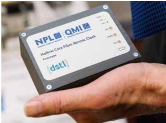
Photonics is at the heart of many of the innovations under development at the UK's four quantum "hubs". The National Physical Laboratory (NPL) is working on new compact atomic clocks that exploit the unusual properties of hollow-core optical fiber. Photo: EPSRC.
