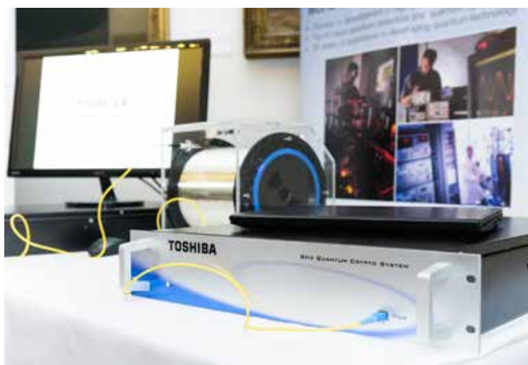
Quantum key distribution (QKD) for highly secure communications is already a commercial, albeit expensive, reality. The UK’s quantum hub based at York is aiming to develop much cheaper versions of the technology and to deploy a secure quantum network in Bristol and Cambridge. Photo: EPSRC.
