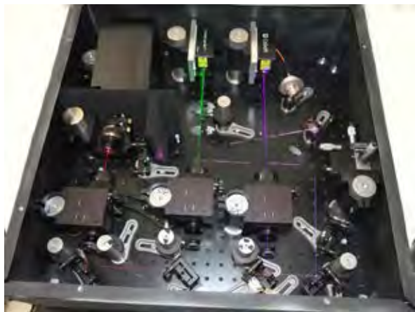
Inside the “ZZZyclops” holographic camera used to capture the Fabergé egg OptoClones , where lasers from Photonics West exhibitor Cobolt provide the key technology.
