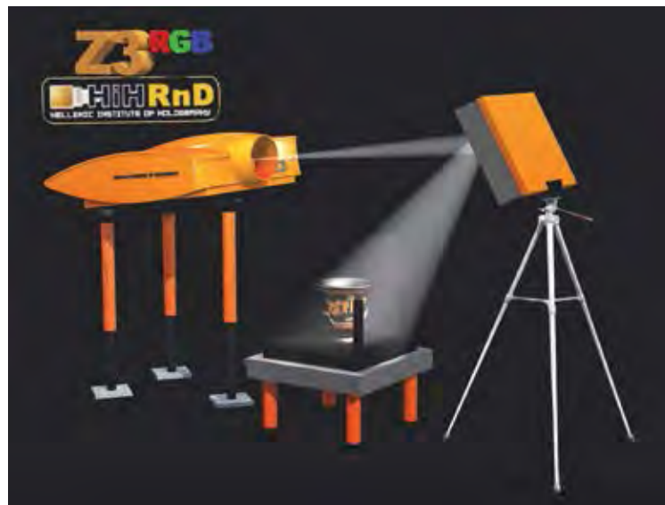
Schematic of the OptoClone recording set-up used to create the ultra-realistic holograms of the Fabergé eggs.
