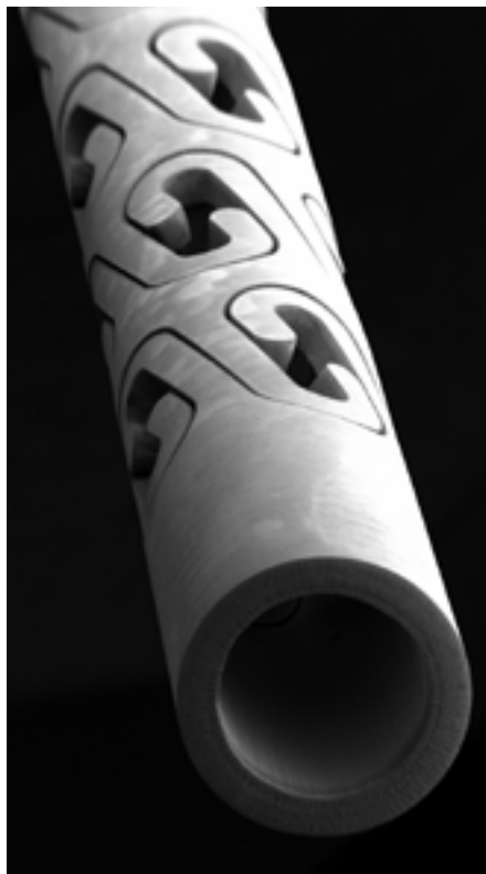
Medical stents, used to aid blood flow in constricted arteries, must be absolutely burr-free. Stents made from the shape-memory alloy nitinol can be precisely machined with an ultrashort pulse laser — eliminating any refinishing work and making their production far cheaper. Credit: TRUMPF Group.
