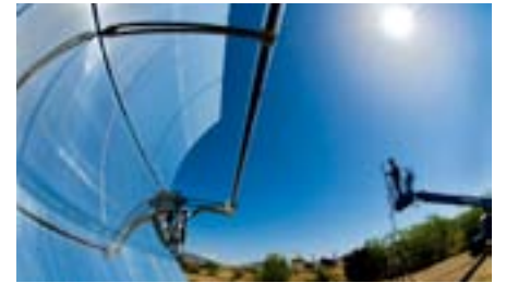
Cranfield’s EPSRC Centre for Innovative Manufacturing in Ultra-Precision has the capability to produce large optical structure such as this solar concentrator, as well as for large telescopes. It hosts a diamond drum-turning facility. Credit: EPSRC/University of Cranfield.
