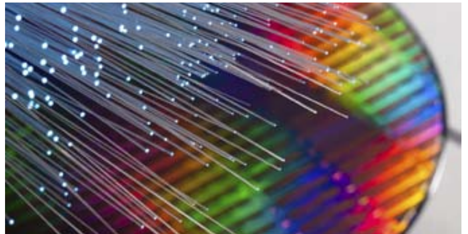
Corning’s “ClearCurve” LX multimode fiber transmits 1310 nm light (the wavelength used by Intel’s silicon photonics modules) at 25 Gb/s with low optical loss, at distances of up to 300 meters — three times further than current technologies. Credit: Corning/Intel.
