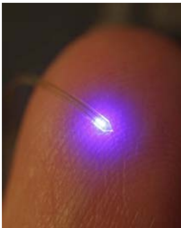
Optogenetics solution? These ultra-miniaturized LEDs devised by the Rogers group are tiny in comparison to commercial devices, and could be used to trigger neurons in the future. Credit: UIUC.
