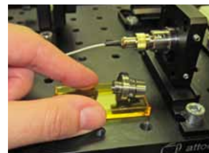
The Attocube sensor measures vibrations at resolution of 1 picometer. A system could range from $20,000 to $60,000. Photo: Ford Burkhart.
