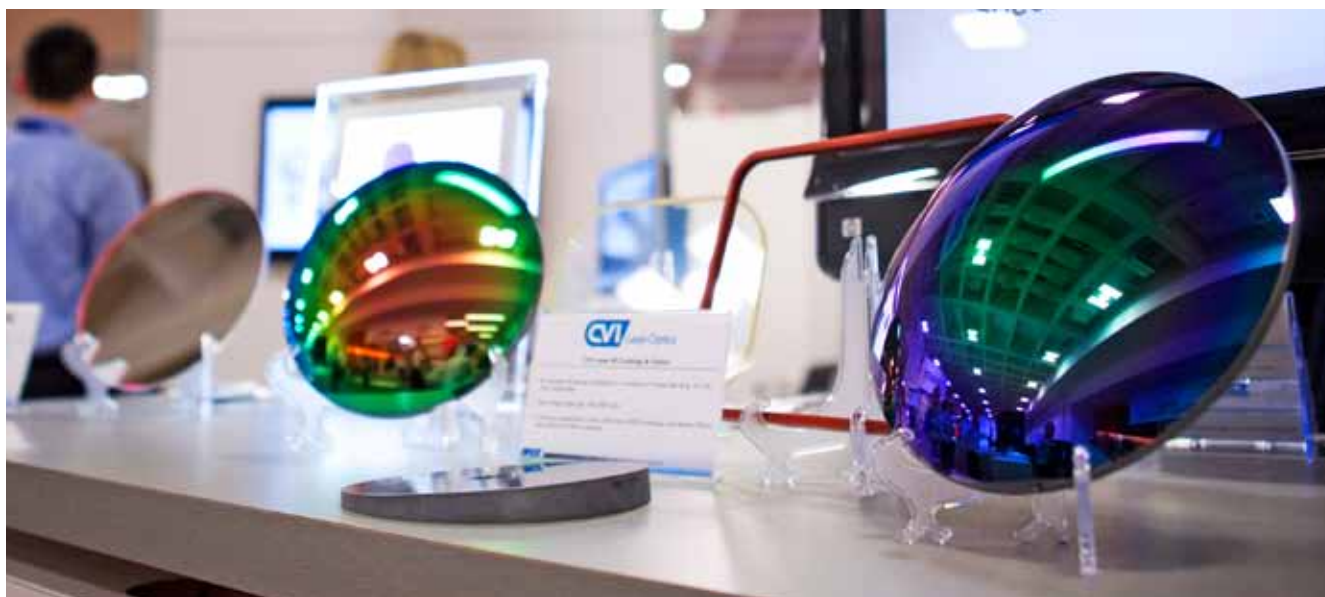
Coated germanium lenses from IDEX’s Semrock subsidiary, on the exhibition floor at Photonics West. The large-scale optics are typically used in defense applications, and the company was highlighting its new 8-inch size thin-film filter (far left), which transmits in the green. Photo: Joey Cobbs
