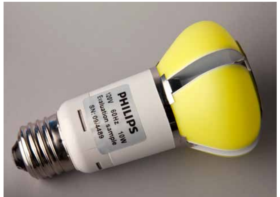
The Philips bulb that won the US Department of Energy’s Lighting Prize draws less than 10 Watts while delivering an output equivalent to a 60W incandescent. It typically retails for about $30, but costs could fall if the bulb could contain fewer LEDs. Understanding the origins of droop could help, because it could allow the deployment of devices driven at far higher currents than those used today, without compromising efficiency. Credit: Philips
