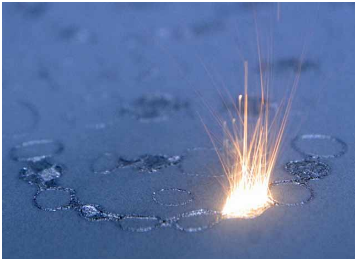
Sparkling smiles: Laser-sintering can be used to make dental crowns and bridges from EOS' CobaltChrome SP2 material. Credit: EOS GmbH
