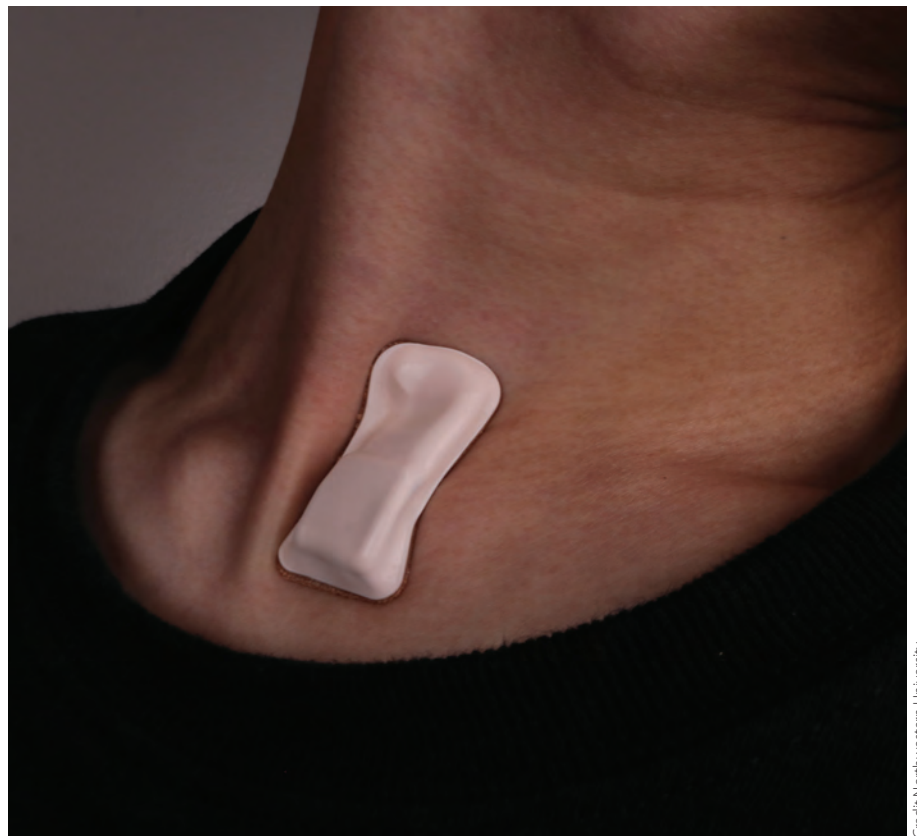
Early warning: the flexible wireless sensor sits on your suprasternal notch to detect Covid-19 symptoms.
