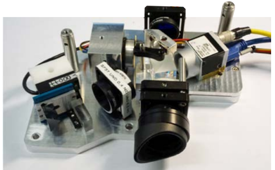
Deep learning has helped to develop an OCT imager for use at home that is smaller and more affordable than standard imagers. Image credit: Gereon Hüttmann/University of Lübeck
