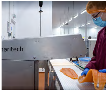
Maritech Eye hyperspectral inspection of salmon.
