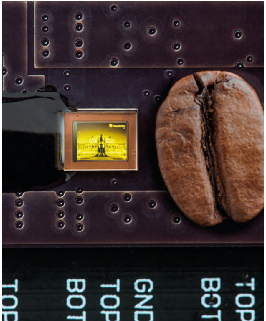
D microdisplay with a resolution of 1440 x 1080 pixels and the world's smallest pixels of 2.5 \mu m.
