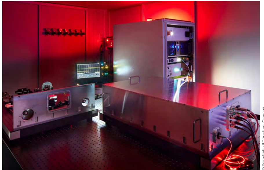
With QuTech, Fraunhofer ILT is developing key components for the quantum internet. Pictured, here, is a laboratory prototype for a low-noise quantum frequency converter.
