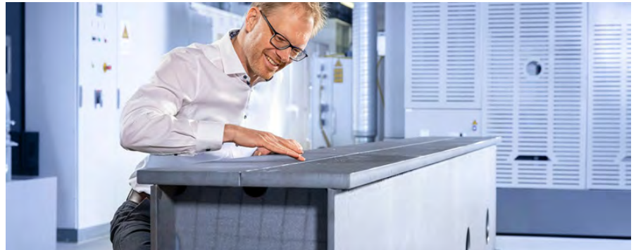
Researchers at the Fraunhofer IWS used an indoor crane segment made of S355J2 structural steel (4 by 0.75 by 0.5 meters) to demonstrate that the laser MPNG welding process they had developed reduces energy costs by up to 80 percent and filler material consumption by up to 85 percent compared to conventional welding processes.
