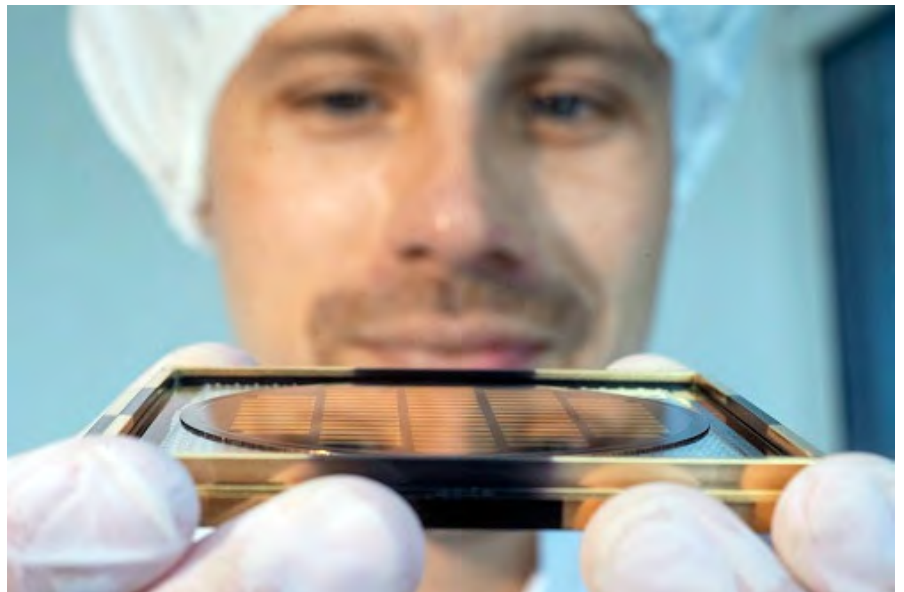
A Q.ANT employee holds up a wafer from which photonic chips are cut.
