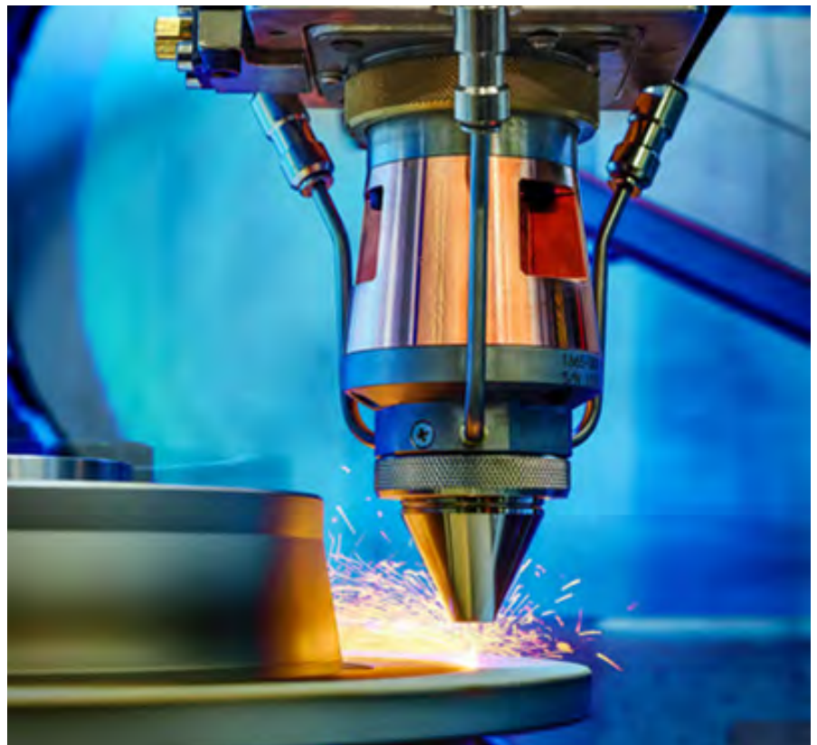
Coating a brake disc with the EHLA process.
