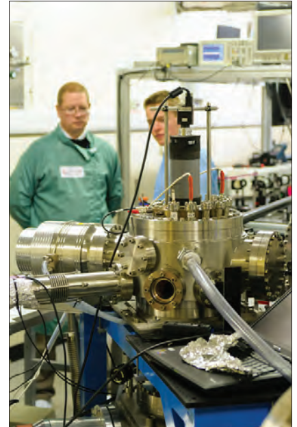
Vacuum apparatus where rotations of complexes were measured.
