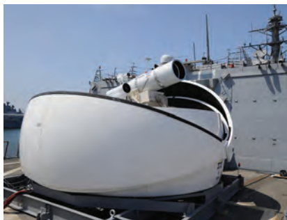
More bang, less bucks: the Laser Weapon System will be installed on USS Ponce.
