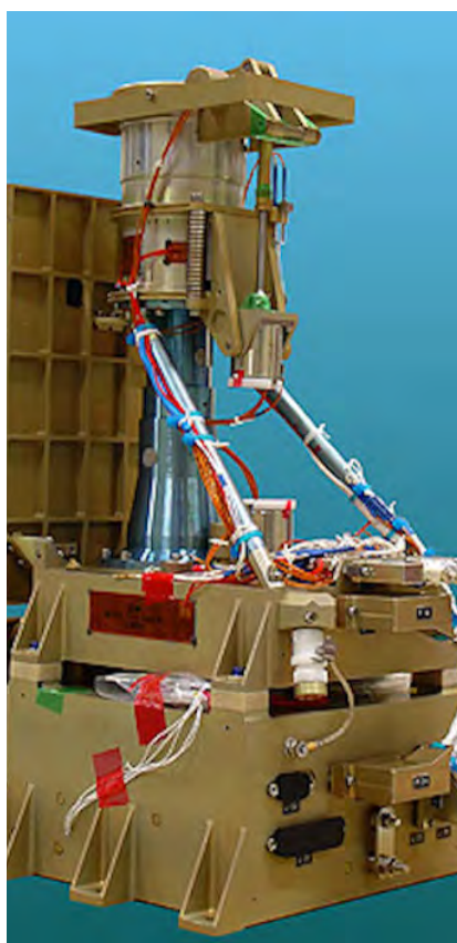
The Asteroid Framing Camera provided to the Dawn mission. Hera is planned to use a flight-spare of the same system.
